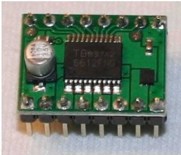
FIG 2. Solder Pololu TB6612FNG Motor Driver Carrier.
