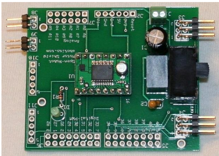
FIG 13. Solder 2x1 Right Angle Connectors, J8 & J9.
