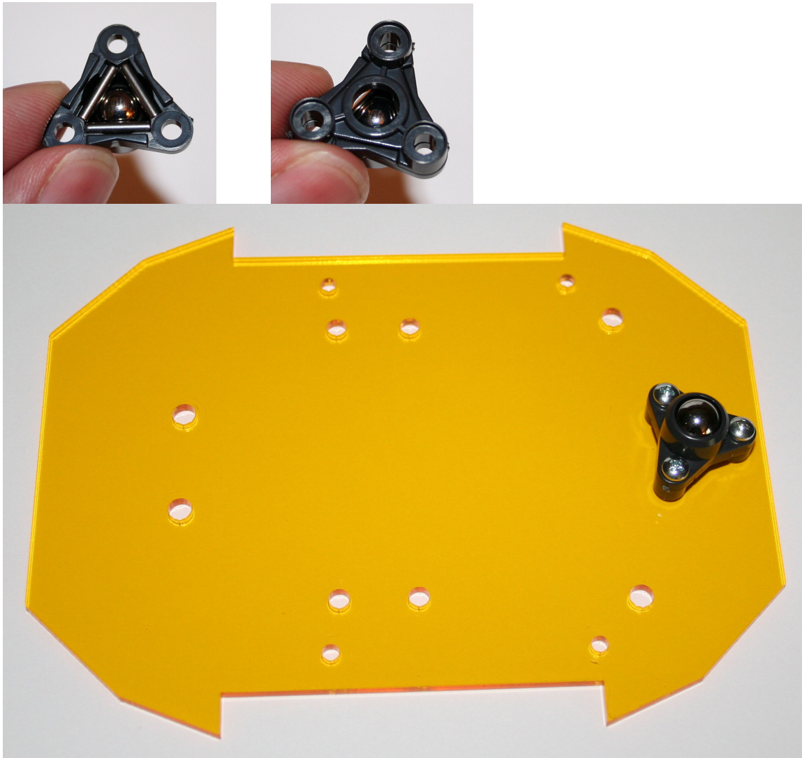
Figure#24, Assemble and mount rear caster wheel.
